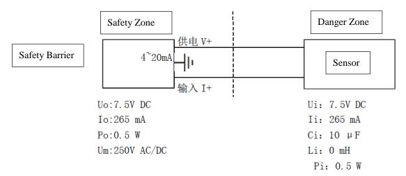
The distribution parameters of the connecting cable between the safety barrier and the sensor should meet:
