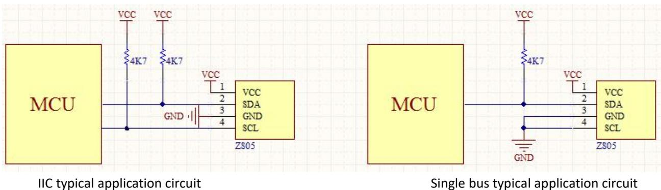
IIC typical application circuit
